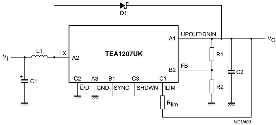
Fig.5 Complete application diagram for upconversion.
