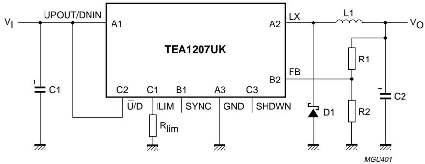
Fig.6 Complete application diagram for downconversion.
