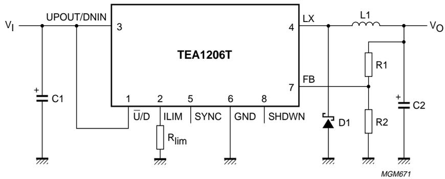
Fig.7 Complete application for downconversion.
