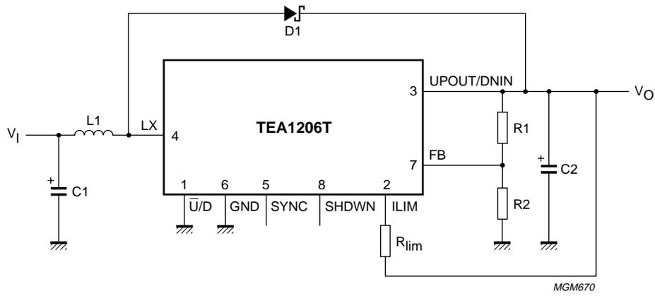
Fig.6 Complete application for upconversion.
