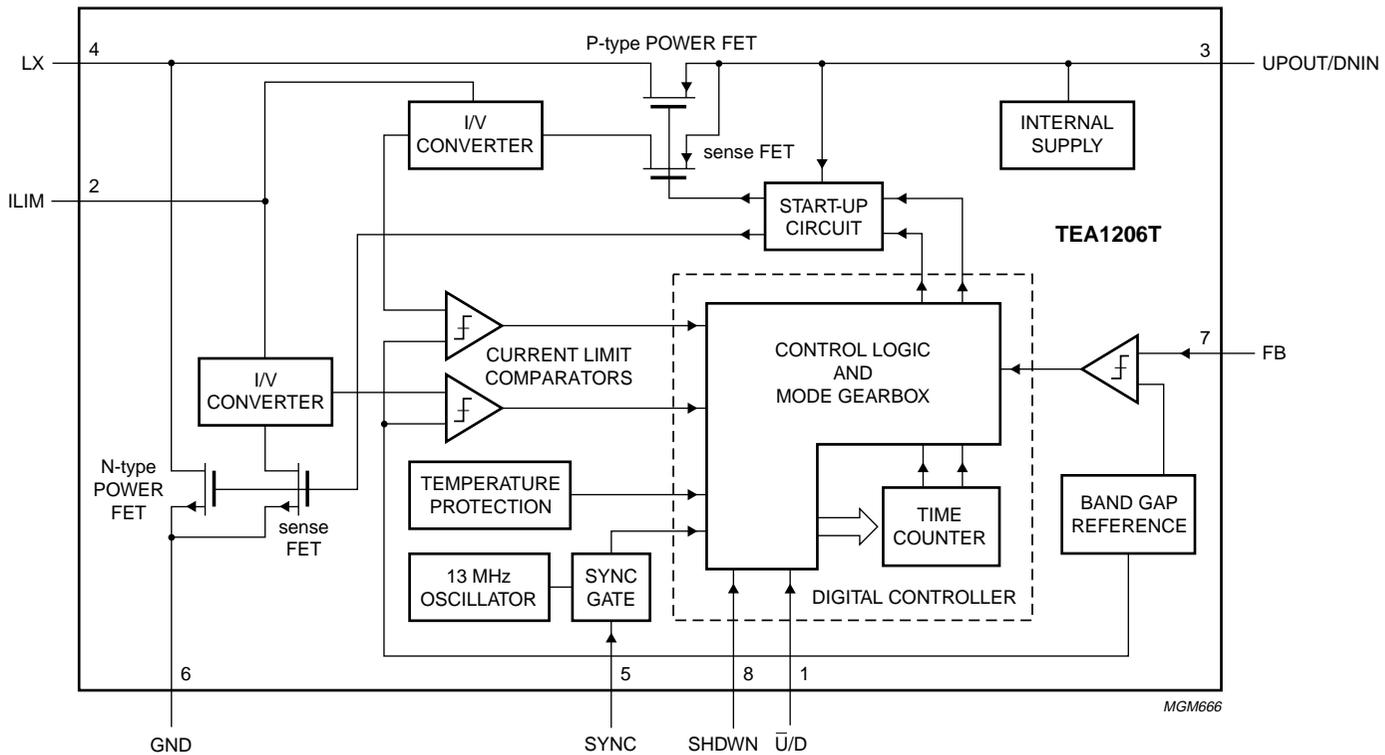
Fig.1 Block diagram.
