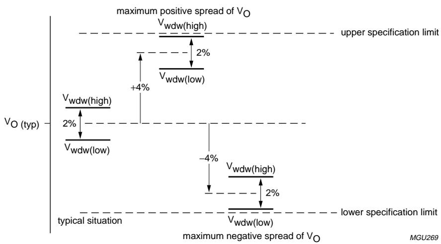
Fig.4 Spread of location of output voltage window.
