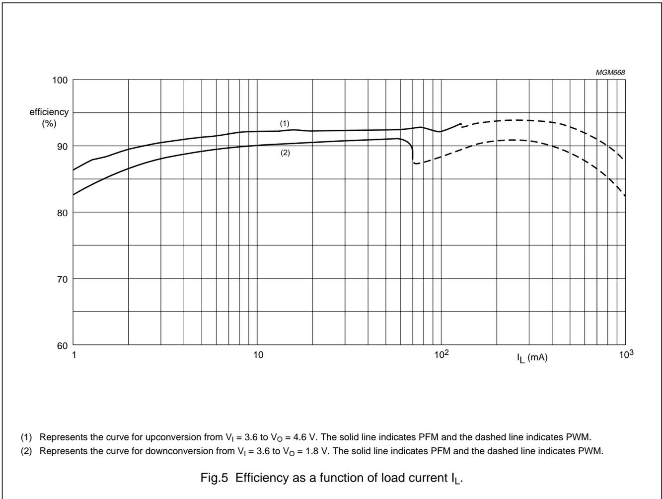
High efficiency DC/DC converter
