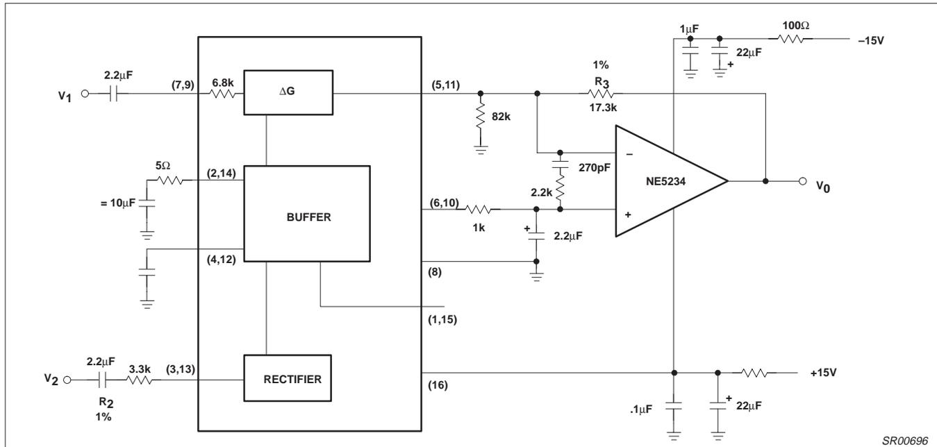
Figure 3. Test Circuit
