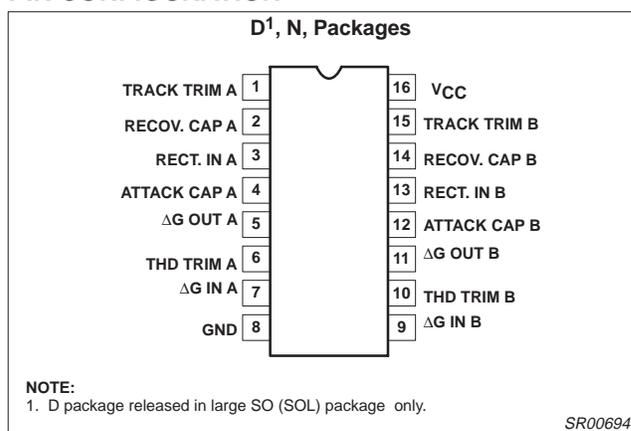
Figure 1. Pin Configuration
