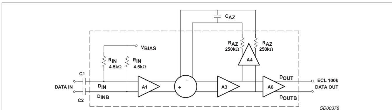
Figure 5. SA5224 Forward Gain Path Including Auto-Zero
