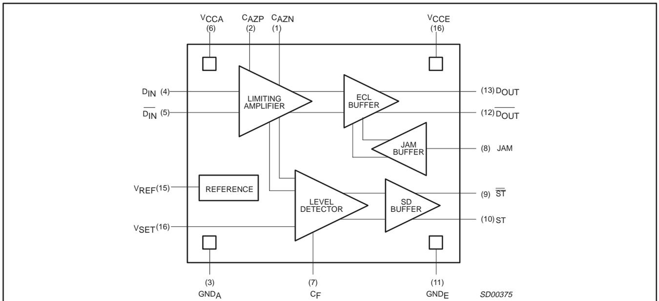
Figure 2. Block Diagram
