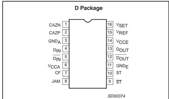
Figure 1. Pin Configuration
