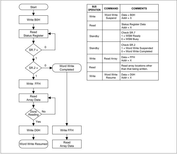
Fig. 6 Word Write Suspend/Resume Flowchart
