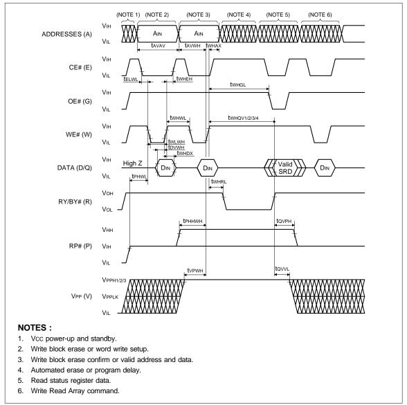
Fig. 12 AC Waveform for WE#-Controlled Write Operations
