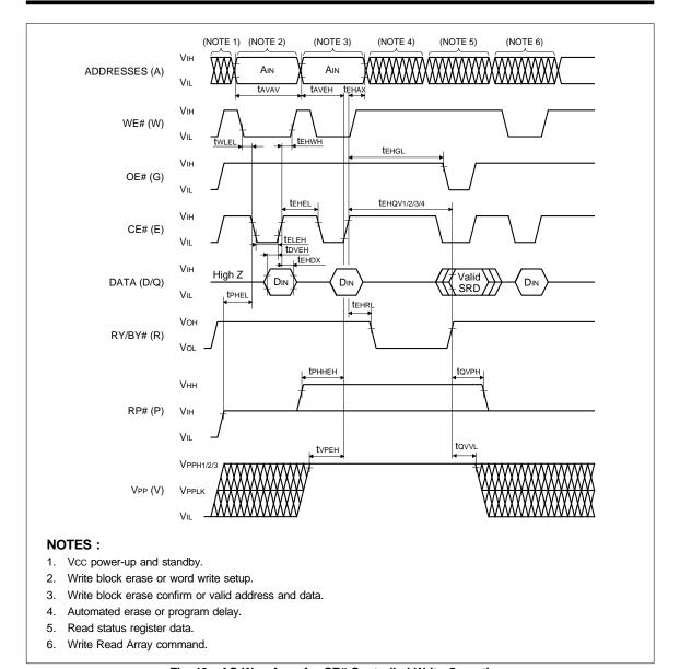
Fig. 13 AC Waveform for CE#-Controlled Write Operations
