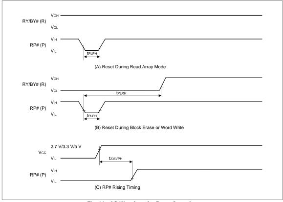
Fig. 14 AC Waveform for Reset Operation
