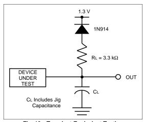
Fig. 10 Transient Equivalent Testing Load Circuit
