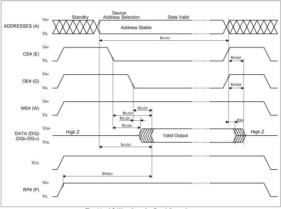
Fig. 11 AC Waveform for Read Operations
