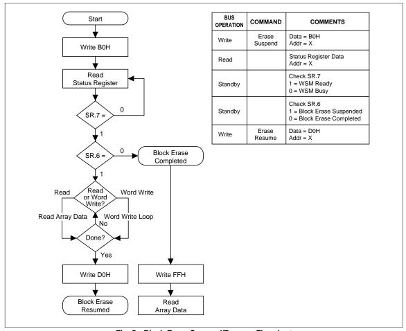
Fig. 5 Block Erase Suspend/Resume Flowchart
