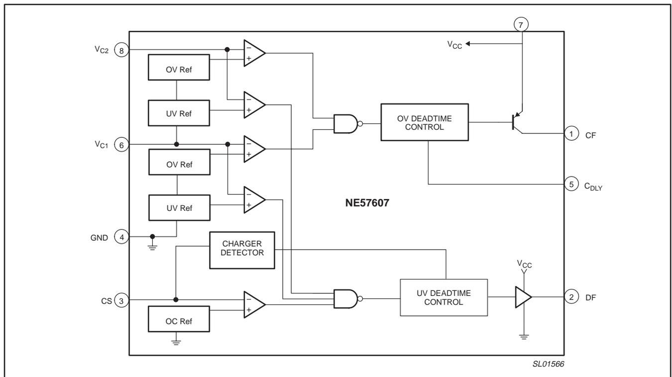
Figure 5. Functional diagram.
