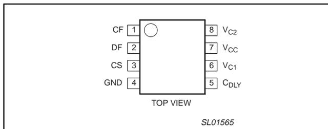
Figure 2. Pin configuration.
