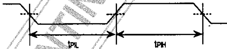
Figure. 6 Pulse input timing condition
