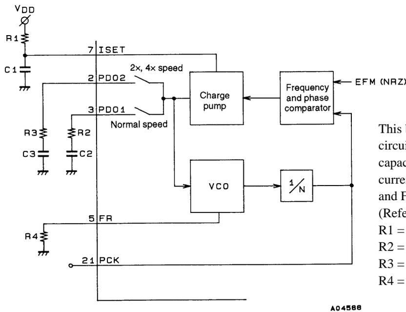
This block includes a VCO circuit, and a PLL circuit is formed using external resistors and capacitors. ISET is the charge pump reference current, PDO1 and PDO2 are the loop filters, and FR determines the VCO frequency range. (Reference values)
