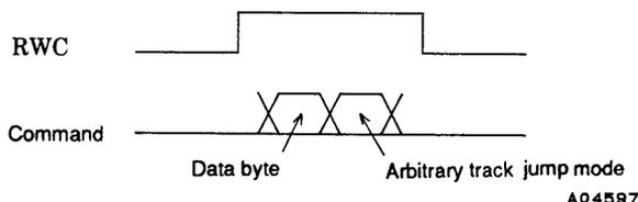
The lower 6 bits of the data byte set the track jump acceleration period (a) and the track jump deceleration period (b). The period a is calculated from the given n and rounded to an integer. The LC78630E monitors the TES half period and terminates the b period if a period longer than the set period elapses.
