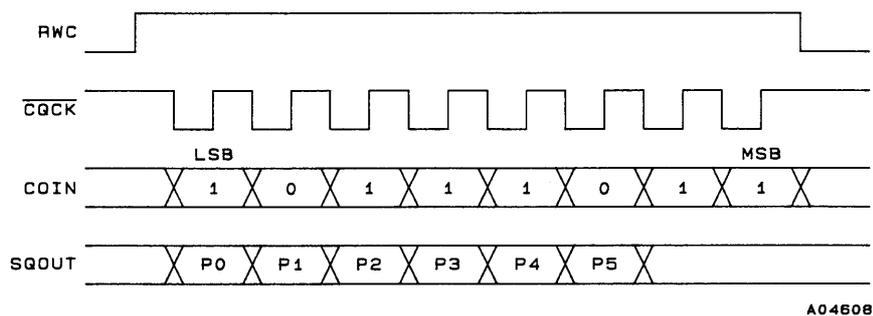
These ports can be set independently to be control output pins by the two-byte port I/O set command. Ports are selected with the lower 6 bits of the data byte.
