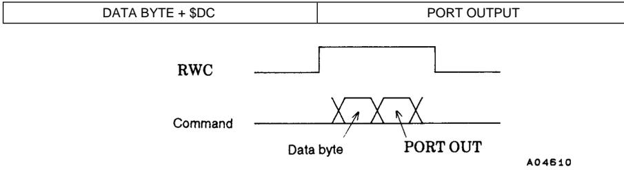
dn = 1 .....A high level is output from Pn, assuming it is set up for output.
