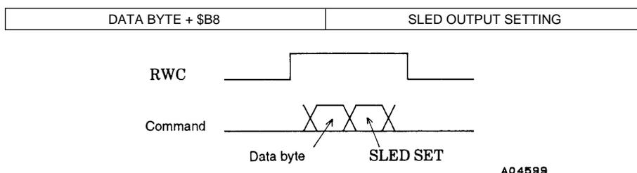
SLED<sup>+</sup> and SLED<sup>-</sup> output is selected by the most significant bit in the data byte. The SLED output level is set by the lower 3 bits. When SLED<sup>+</sup> is set, SLED<sup>-</sup> is automatically set to V<sub>SS</sub> (SLED off). The inverse is also true.
