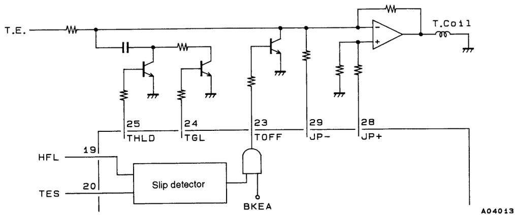
When the LC78630E is used in combination with a LA9230/40 Series LSI, since the THLD signal is generated by the LA9230/40 Series LSI, the THLD pin (pin 25) will be unused, i.e., have no connection.
