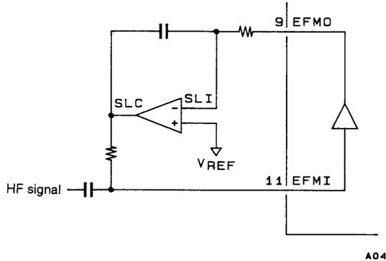
When an HF signal is input to EFMI, the circuit slices it at an optimal level to produce an EFM (NRZ) signal.
