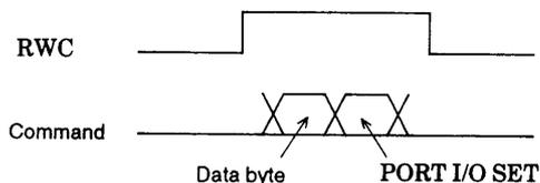
dn = 1 .....Sets port Pn to be an output pin.
