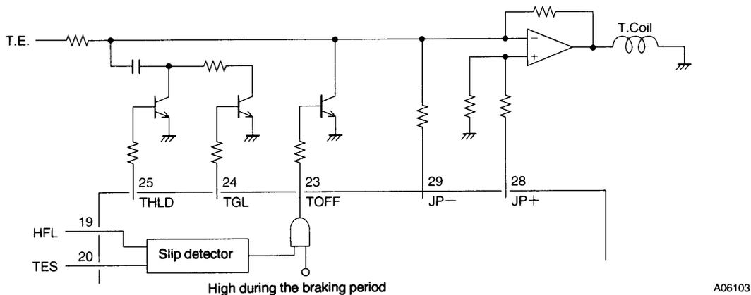
When the LC78625E is used in combination with an LA9230/40 Series LSI, since the THLD signal is generated by the LA9230/40, the THLD pin (pin 25) will be unused, and should be left open.
