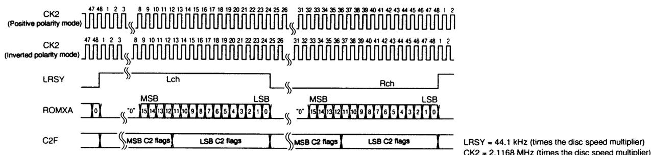
21. Digital output circuit; Pin 56: DOUT
