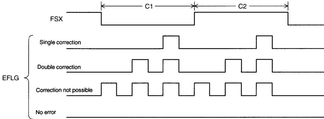
The FSX signal is generated by dividing the crystal oscillator clock, and is a 7.35 kHz frame synchronization signal. The error correction state for each frame is output from EFLG. The playback OK/NG state can be easily determined from the extent of the high level that appears here.
