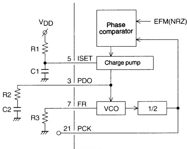
Since the LC78625E includes a VCO circuit, a PLL circuit can be formed by connecting an external RC circuit. ISET is the charge pump reference current, PDO is the VCO circuit loop filter, and FR is a resistor that determines the VCO frequency range.
