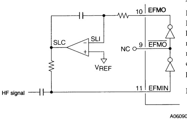
The LC78625E handles defects as follows. When a high level is input to the DEFI pin (pin 1), the  $\overline{\text{EFMO}}$  (pin 9) and EFMO (pin 10) pins (the slice level control outputs) go to the high-impedance state, and the slice level is held. However, note that this function is only valid in CLV phase control mode, that is, when the V/P pin (pin 15) is low. This function can be used in combination with the LA9230/40 series DEF pin.
