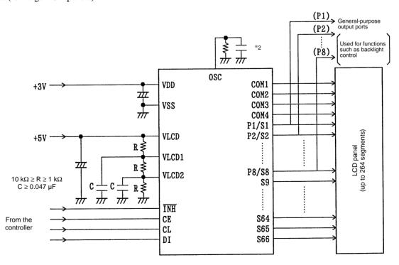
Note: \*2 When a capacitor except the recommended external capacitance (Cosc = 680 pF) is connected the OSC pin, we recommend that applications connect the OSC pin with a capacitor in the range 220 to 2200 pF.
