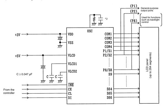
Note: \*2 When a capacitor except the recommended external capacitance (Cosc = 680 pF) is connected the OSC pin, we recommend that applications connect the OSC pin with a capacitor in the range 220 to 2200 pF.
