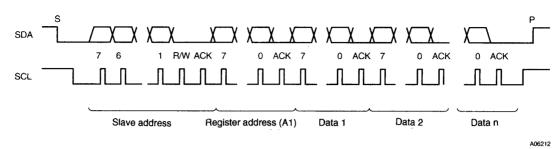
Data 1 is stored at register address A1. Data 2 is stored at register address A1 + 1, i.e., the address given by incrementing A1. If the address exceeds 11H, it wraps to 00H.
