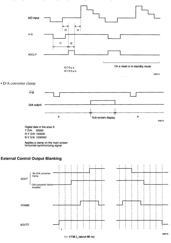
Note: FRAME is only output when there is not D/A converter frame.
