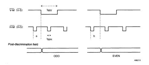
The periods a and b must be in the following ranges: a=0.02 to 0.40 H b=0.60 to 0.98 H The synchronizing signal pulse widths must meet the following conditions:  $t_{WV}>1~\mu s$  $t_{WH}>1~\mu s$
