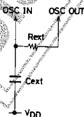
Fig. 11 Recommended CR oscillation circuit
