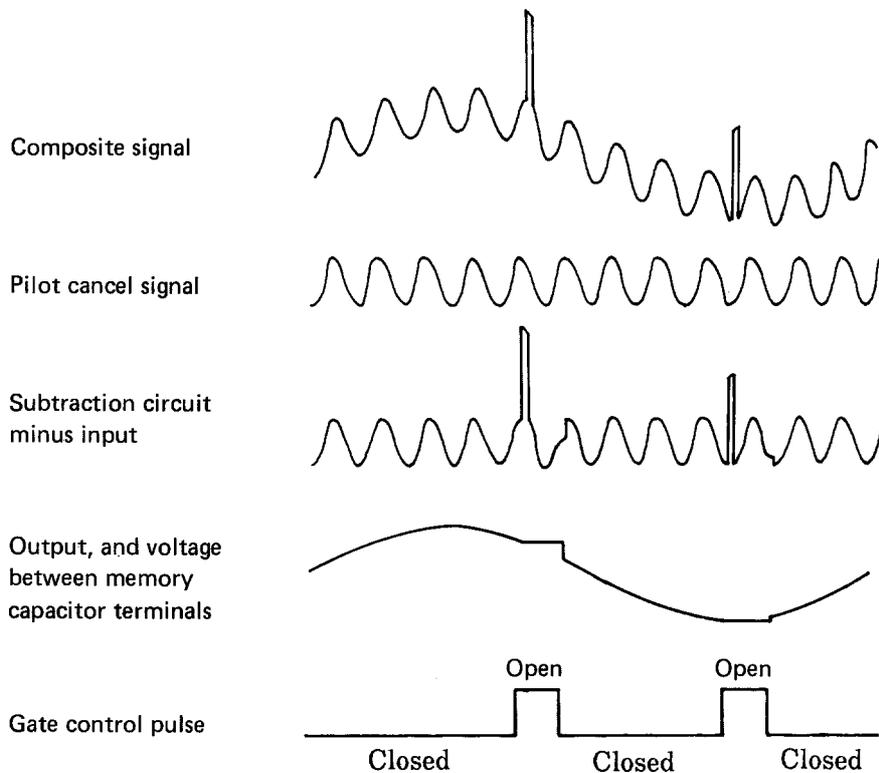
Note : The pilot cancel signal is given as sinusoidal in this explanation, but in the actual application circuit, pilot cancel is performed by a triangular wave.
