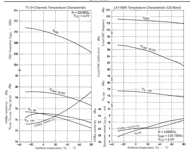
(Note) 65dBμ sensitivity : Input at 65 dBμ in Temperature Characteristic Test Circuit
