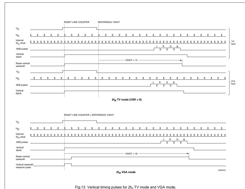
C-bus controlled TV display processors
