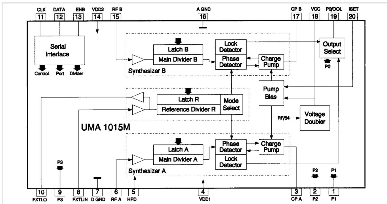
Figure 1. UMA1015M Dual Synthesizer for Mobile Radio Communications
