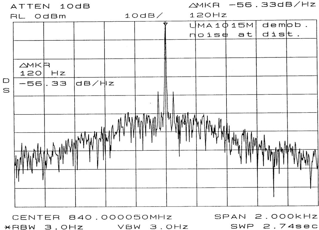
Figure 11. UMA1015M Demoboard, Frequency Spectrum Synthesizer B, 2kHz Span. Close-in Noise: 56dB/Hz Below Carrier.
