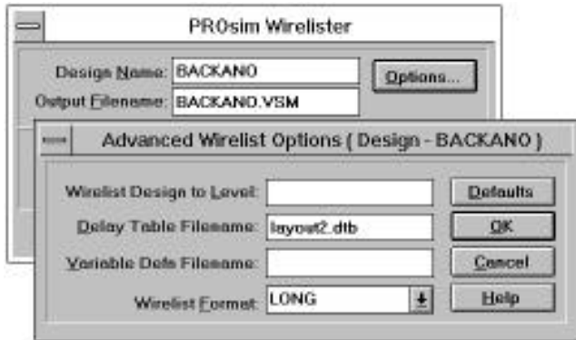
Figure 10. VSM Netlister, and its Options sub-window. "BACKANO" is the design name. The back annotation file name is "layout2.dtb".
