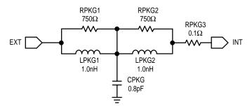
Figure 4. Package Model Schematic
