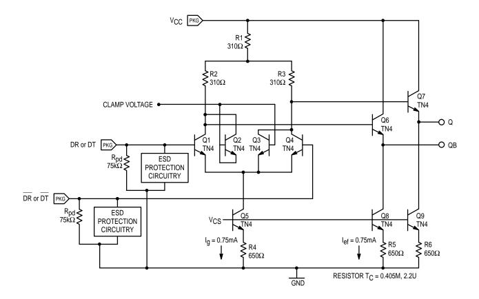
Figure 1. Simplified Input Schematic
