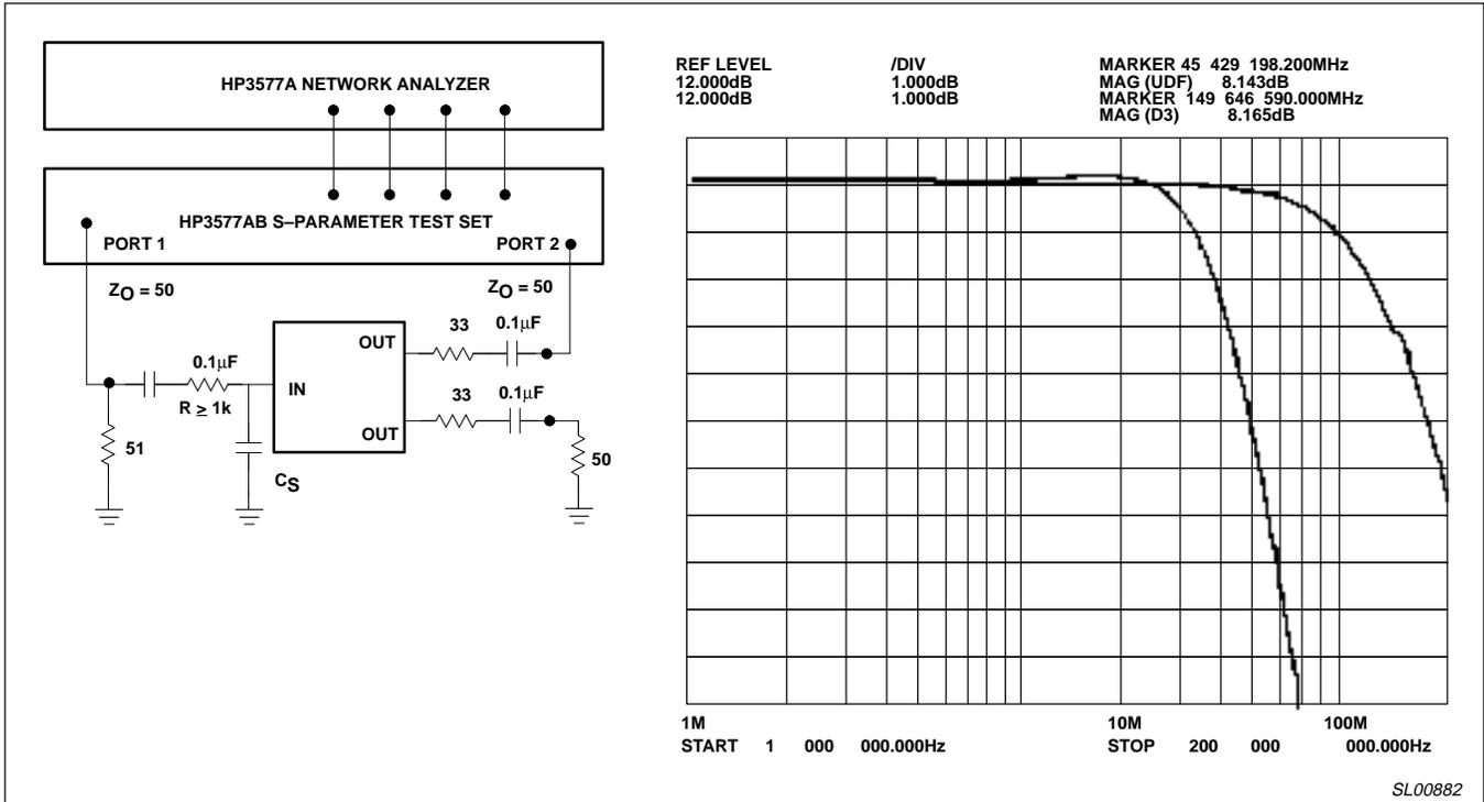
Figure 13. Setting Bandwidth with Shunt Input Capacitor, C<sub>S</sub>
