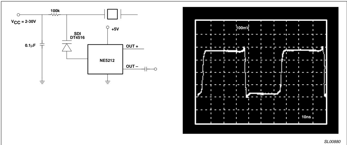
Figure 11. Varactor Tuned Crystal Oscillator with 0.28% Tuning Range
