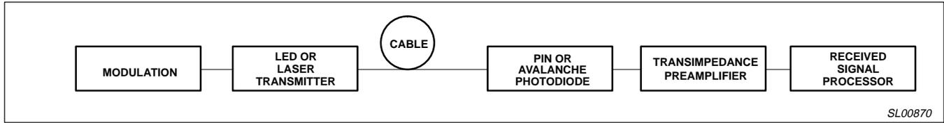
Figure 1. Fiber Optic Transmission System Using Transresistance Preamplifier
