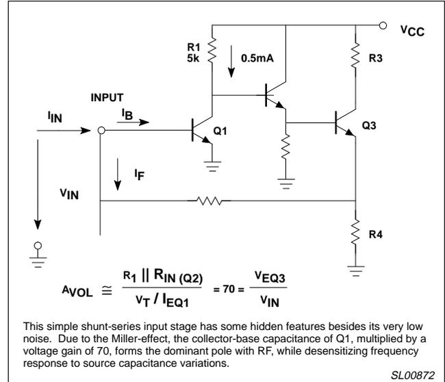
This simple shunt-series input stage has some hidden features besides its very low noise. Due to the Miller-effect, the collector-base capacitance of Q1, multiplied by a voltage gain of 70, forms the dominant pole with  $R_F$ , while desensitizing frequency response to source capacitance variations.
