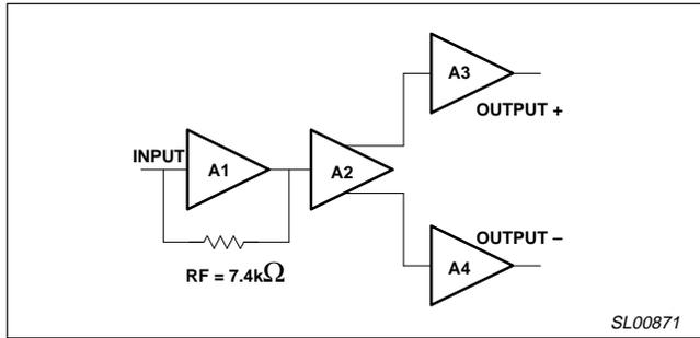
Figure 2. NE5212 Block Diagram Showing the Transresistance Preamplifier with the Internal Feedback Resistor and the Buffered Differential Outputs.
