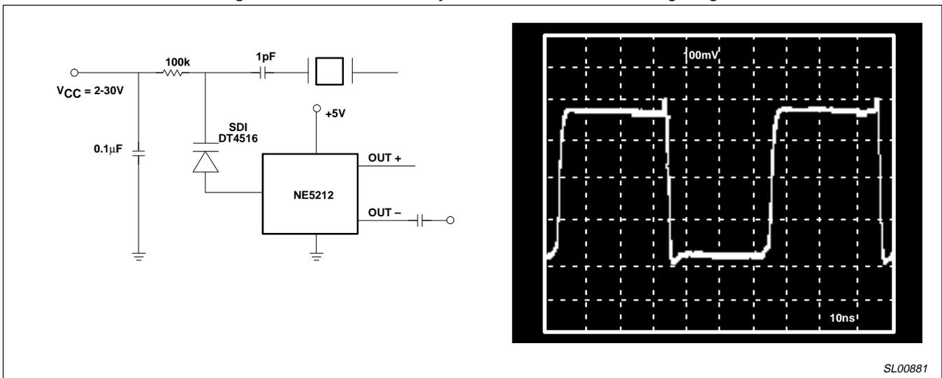
Figure 12. Varactor Tuned Oscillator with 1ppm/V Supply Sensitivity
