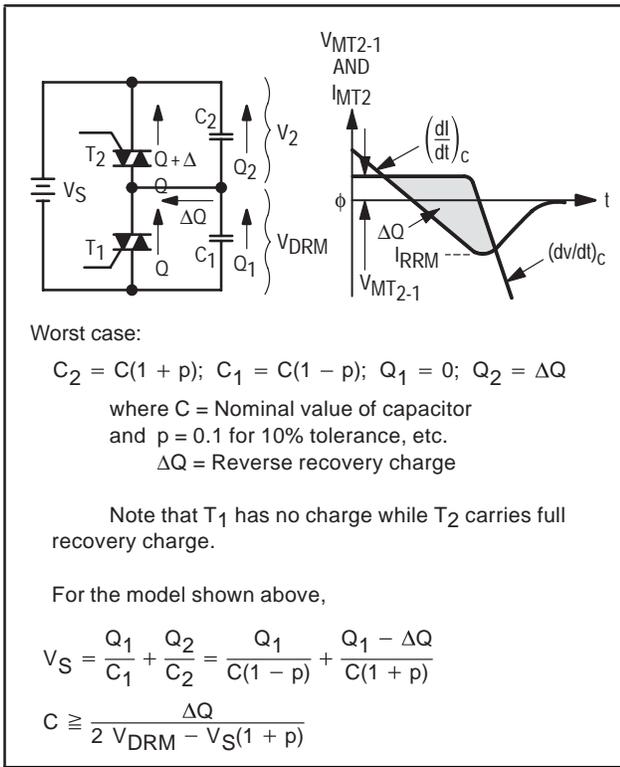
Figure 6.12. Minimum Capacitor Size for Dynamic Voltage Sharing
