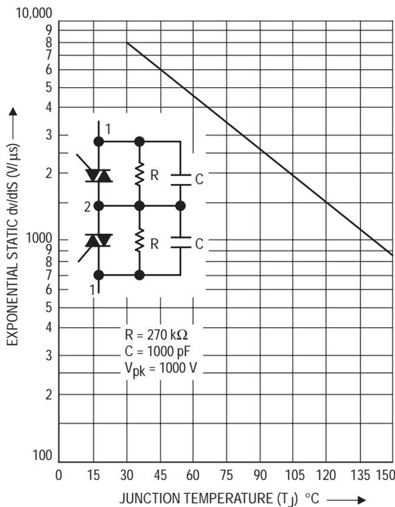
**Figure 6.9. Exponential Static dV/dt, Series MAC15-8 Triacs**
