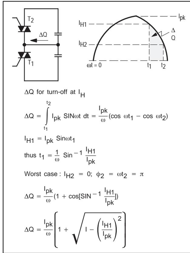
Figure 6.14. Forward Recovery Charge for Turn-Off at  $I_H$
