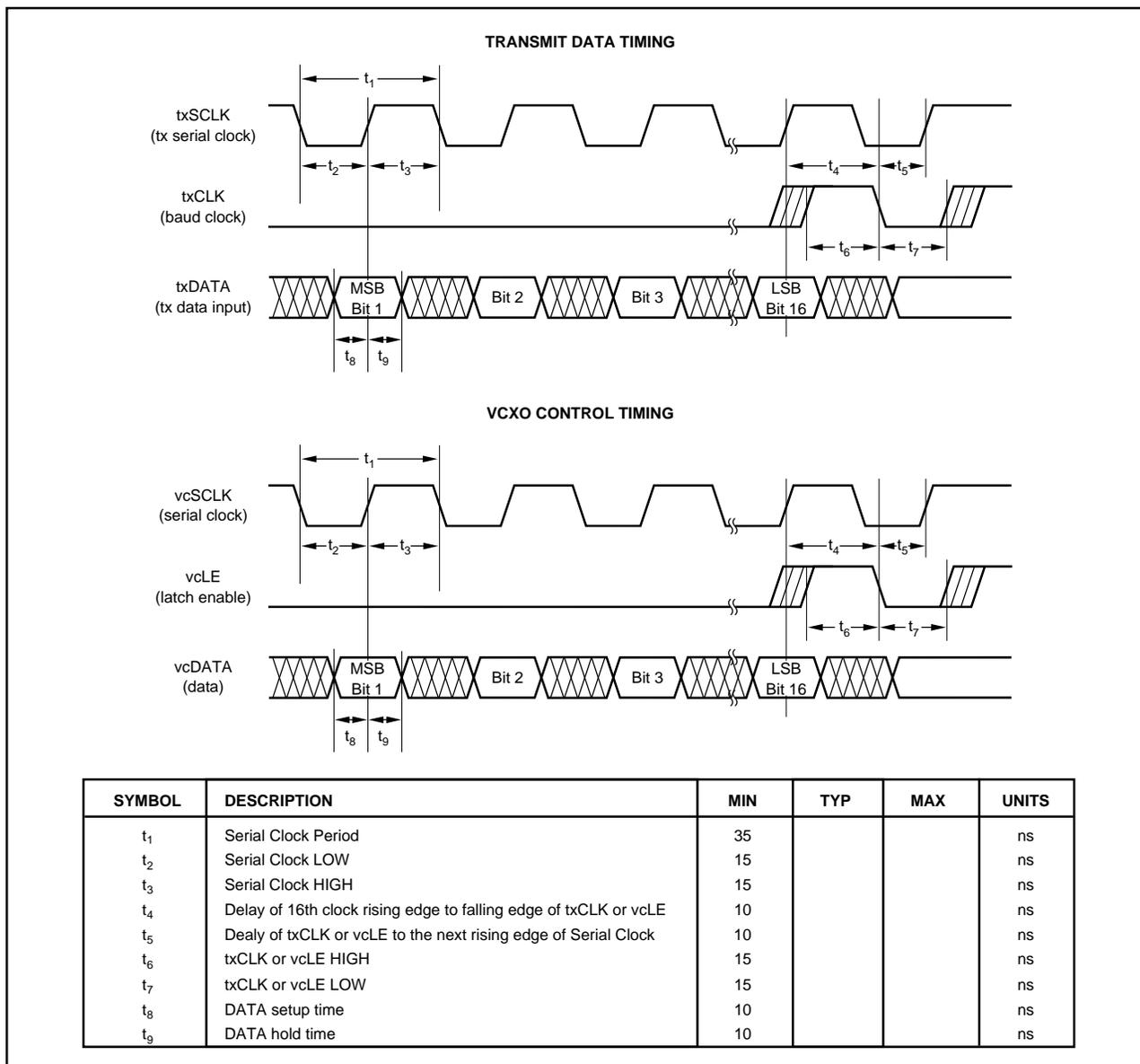
FIGURE 4. Timing Diagram.
