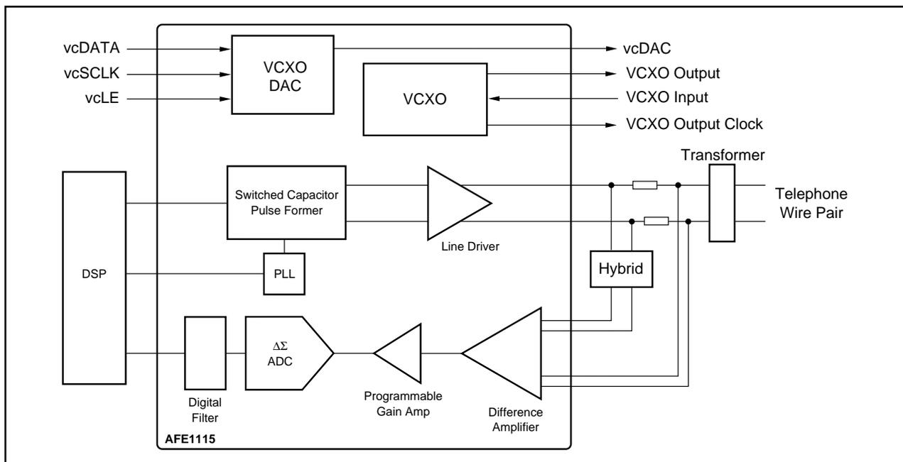
FIGURE 1. Functional Block Diagram of AFE1115 Circuit.
