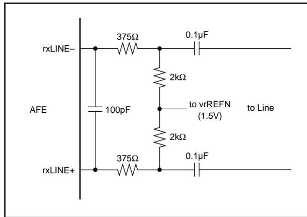
FIGURE 3. Optional rxLINE Input Common-mode Voltage Control.
