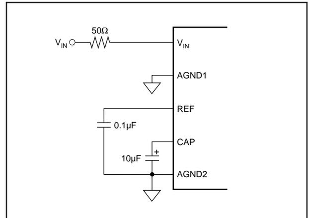
FIGURE 4b. Circuit Diagram Without External Hardware Trim.
